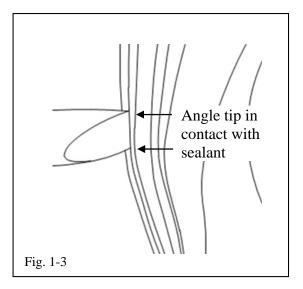
Align the adjustment tool to the edge of the door, with the angle edge positioned toward the inside of the door (Fig. 1-3).
